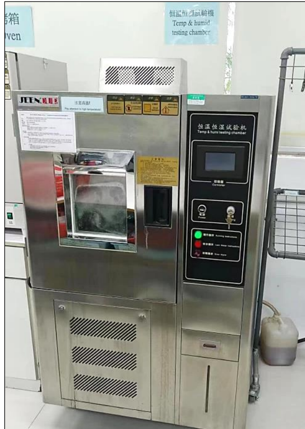
Ageing Test under hot humid condition (70 °C, RH 90%, 7dys)
